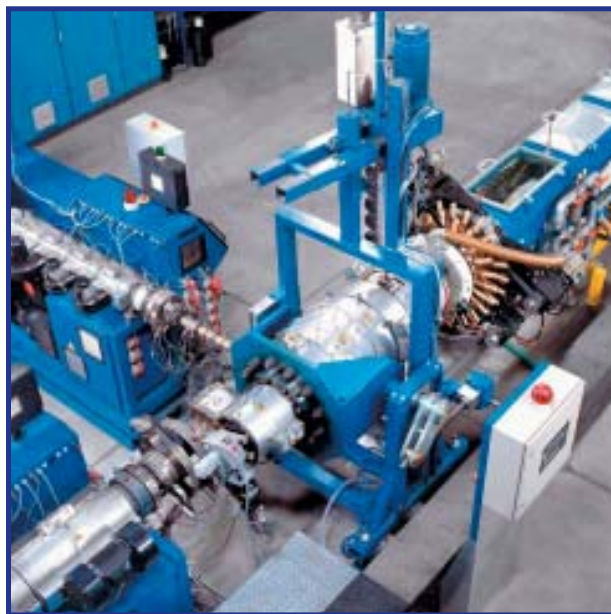
QuickSwitch pipe extrusion system enables the diameter and wall thickness to be changed "on the fly." Krauss-Maffei.
